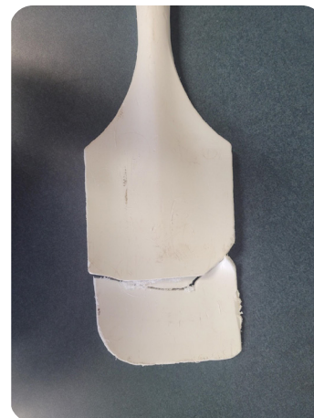
Attached image of the paddle pieced together to determine if/show evidence all pieces are accounted for.
